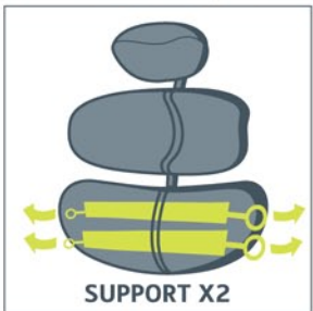
SUPPORT X2 The 2 internal straps of each segment provide adjustable lumbar profile
